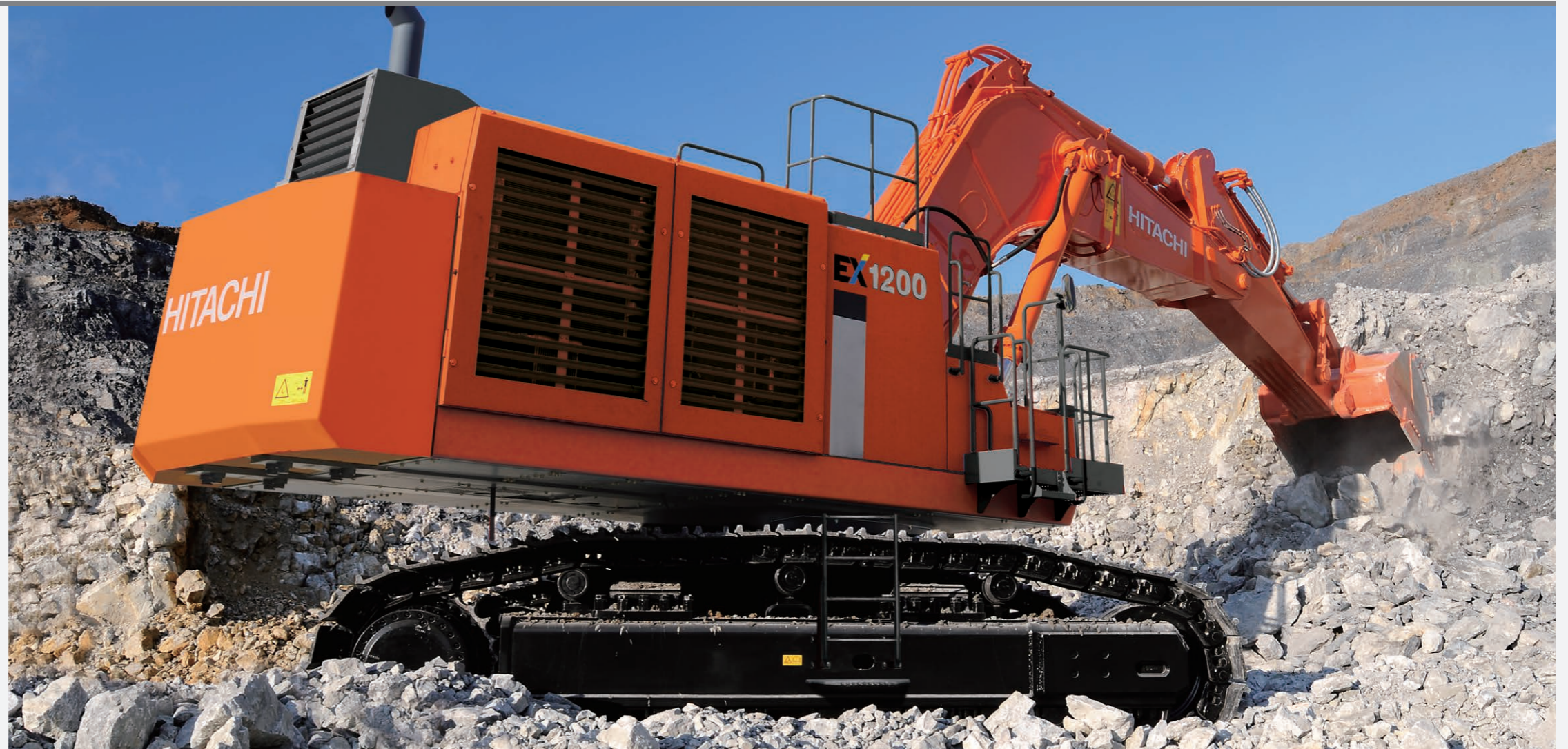
Notes : This photo includes custom-designed components, including reinforcing plates for side track frame.
