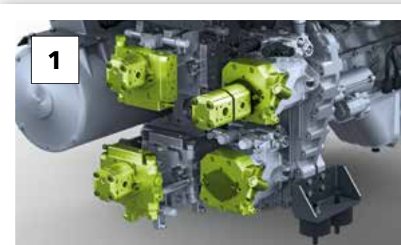
Splitter gearbox with ability to disengage hydraulic pumps
